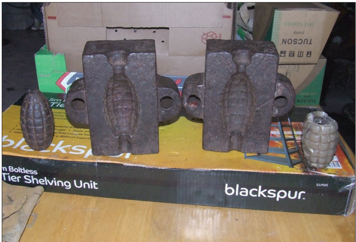
Plate 5. Grenade moulds and 'blank' grenades from Ballynanelagh Bomb Factory.
