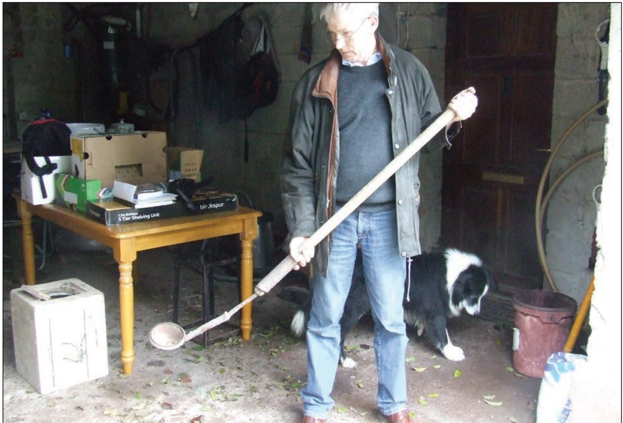
Plate 6. The 'crucible' used for molten metal and fabricated out of an old kettle, now with replacement handle. Used in Ballynanelagh Bomb Factory.
